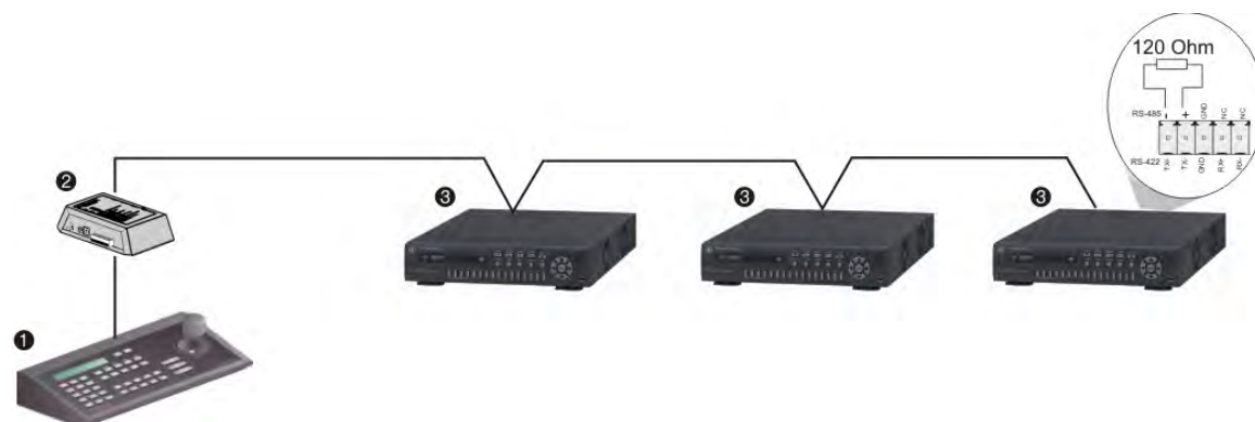
Figure 6: RS-485 bus serial wiring
