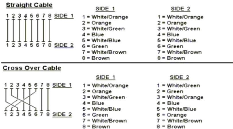
Figure A-1: Straight-Through and Crossover Cable
