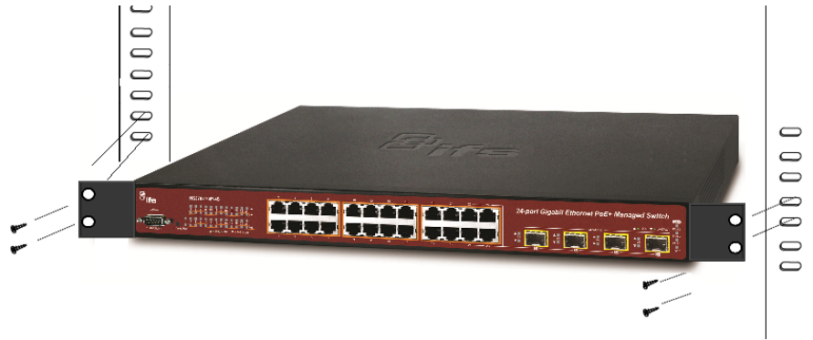
Figure 2-2-3: Mounting Managed Switch in a Rack
