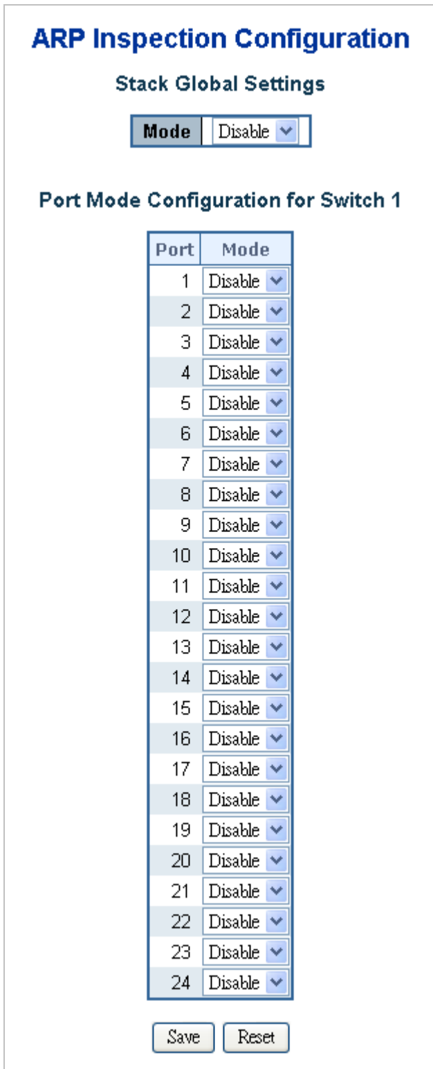
Figure 4-12-12 ARP Inspection Configuration screen page screenshot
