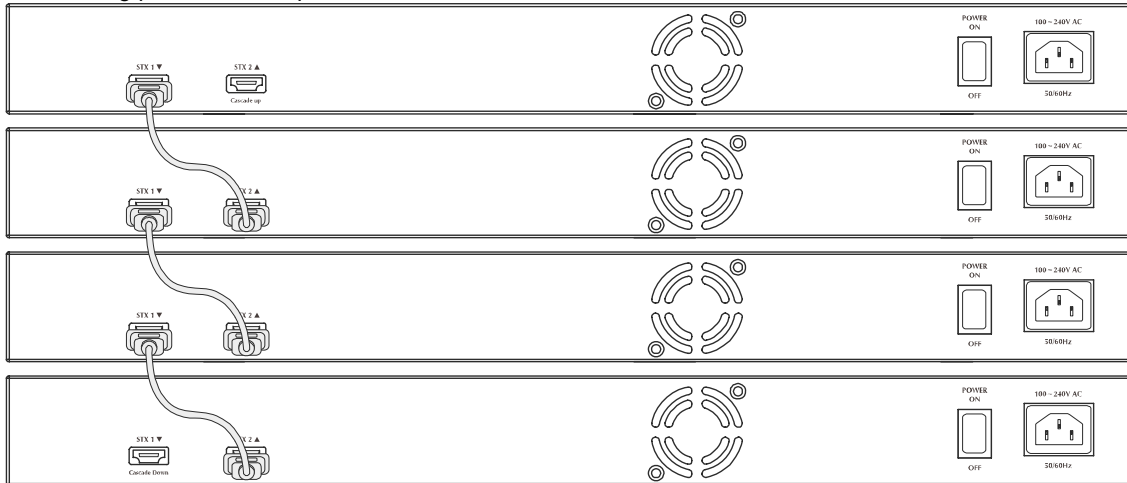
Figure 2-11 Chain Stack topology
