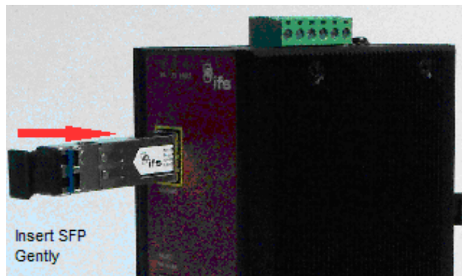
Figure 2-5: Plug-in the SFP Transceiver
