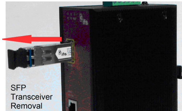
Figure 2-6: Pull Out the SFP Transceiver Module
