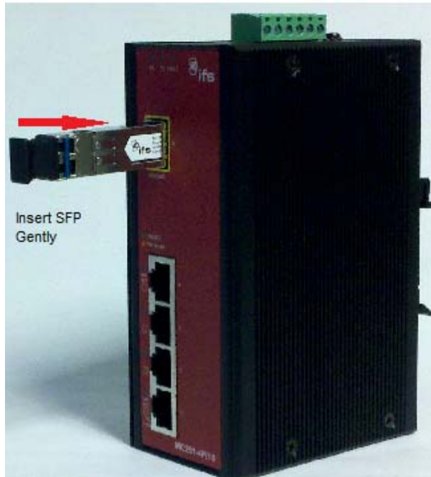
Figure 2-9: Plugging in the SFP Transceiver
