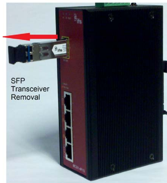
Figure 2-10: How to Pull Out the SFP Transceiver Module
