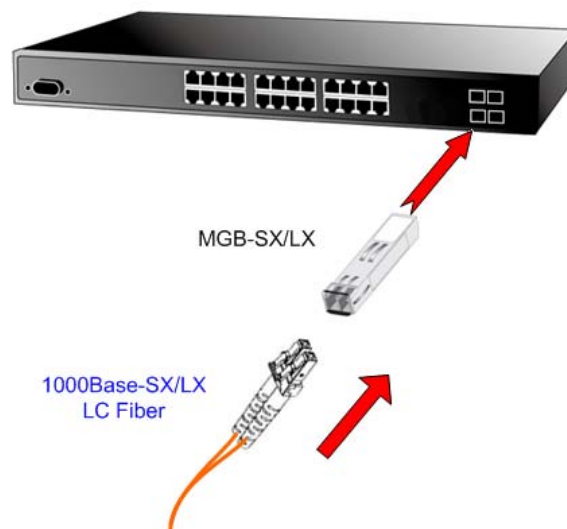
Figure 2-7 Plug-in the SFP Transceiver
