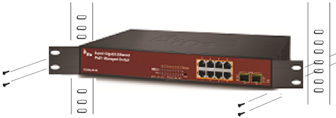
Figure 2-6: Mounting NS3502-8P-2S in a Rack
