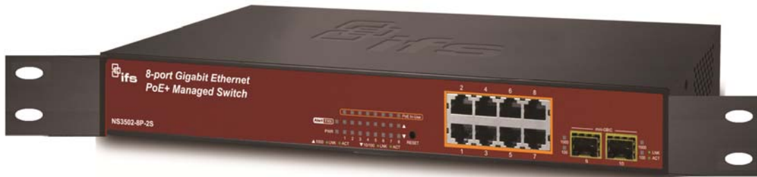
Figure 2-5: Attach brackets to the Managed Switch.
