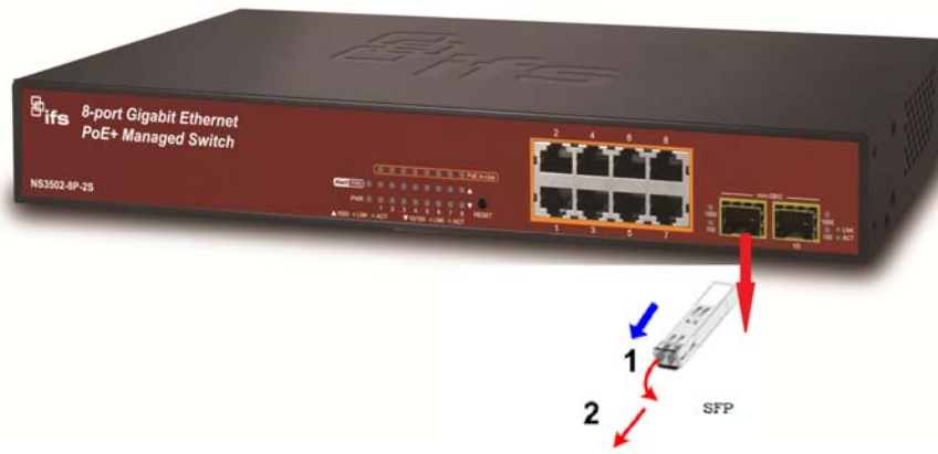
Figure 2-8: Pull out the SFP transceiver
