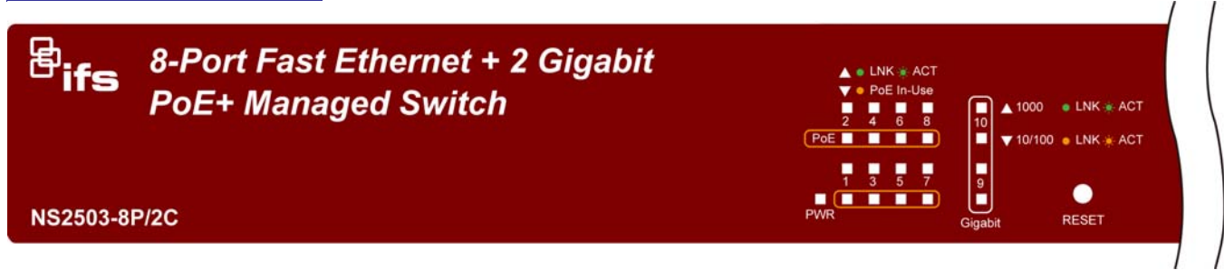
Figure 2-6: NS2503-8P/2C LED panel
