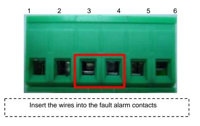
**Note:** The wire gauge for the terminal block should be in the range between  $12 \sim 24$  AWG.
