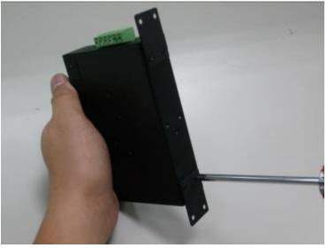
3. Assemble the wall mount plate on the MC251-4P/1S and the NS2051-4P/1T.
