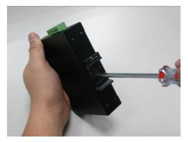
2. Place the wall mount plate on the rear panel of the MC251-4P/1S and the NS2051-4P/1T.
