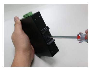
2. Place the wall mount plate on the rear panel of the MC250-4T.
