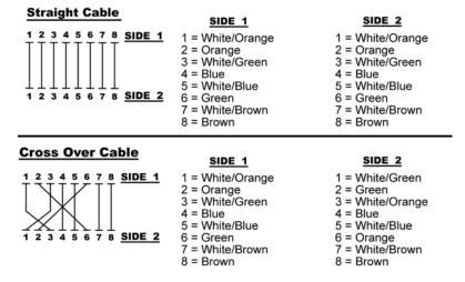
Please make sure your connected cables are with same pin assignment and color as above picture before deploying the cables into your network.
