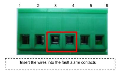
**Note:** The wire gauge for the terminal block should be in the range between 12 ~ 24 AWG.
