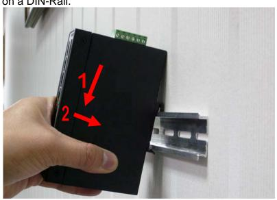
1. Lightly press down and push the bottom of the DIN-Rail connector mount into the track.
