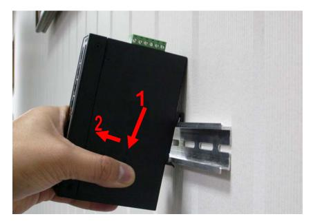
4. Lightly press down and pull the bottom of DIN-Rail connector mount to remove it from the track.
