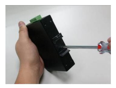
2. Place the wall mount plate on the rear panel of the MC250-1T/1S.
