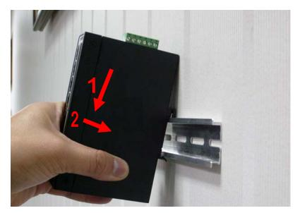
1. Lightly press down and push the bottom of the DIN-Rail connector mount into the track.
