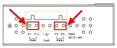
2. Tighten the wire-clamp screws to prevent the wires from disconnecting.
