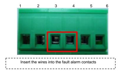
**Note:** The wire gauge for the terminal block should be in the range between  $12 \sim 24$  AWG.
