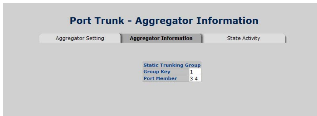
Figure 5-22: Static Trunking Group information
