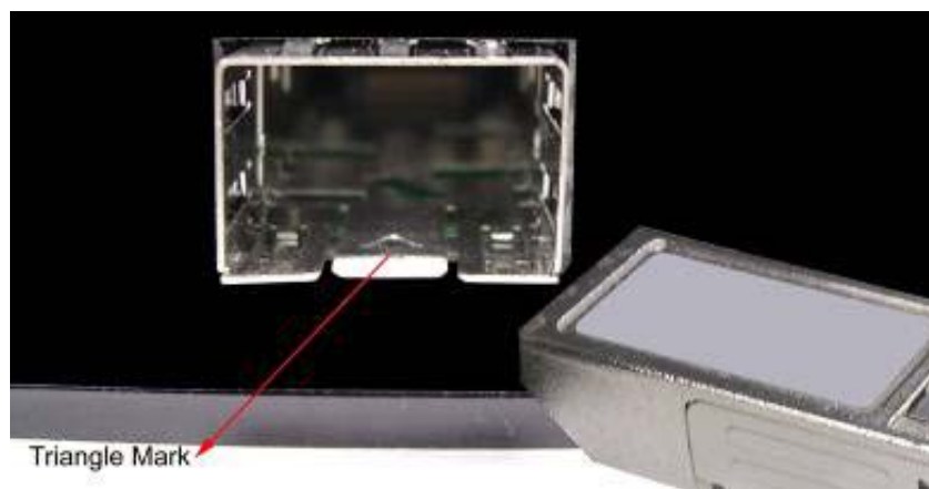
Figure 2-19: Plug-in the SFP transceiver
