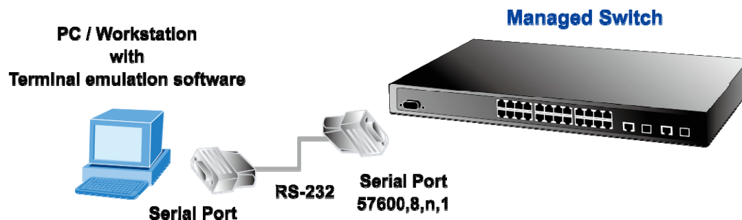
Figure 3-4: Console management setup
