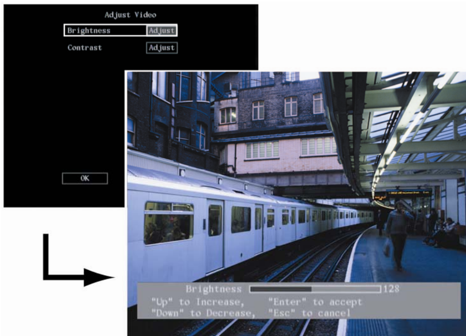
Figure 28: The Brightness option in the camera Adjust Video submenu
