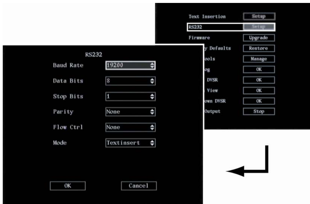
Figure 61: The RS-232 submenu
