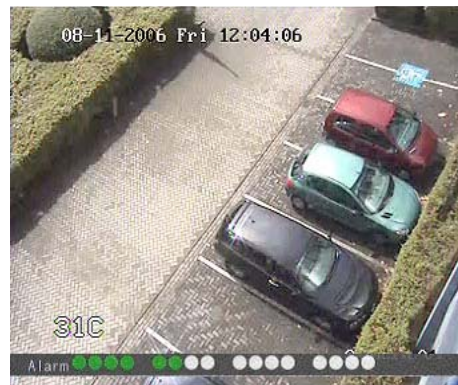
Figure 5: Alarm status in live viewing mode (16-channel system shown)
