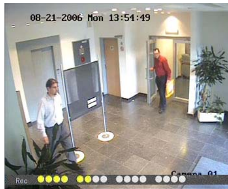
Figure 4: Record status in live viewing (Preview) mode (16-channel system shown)
