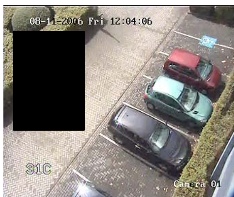
Figure 22: Example of a masked area in the mark area setup screen
