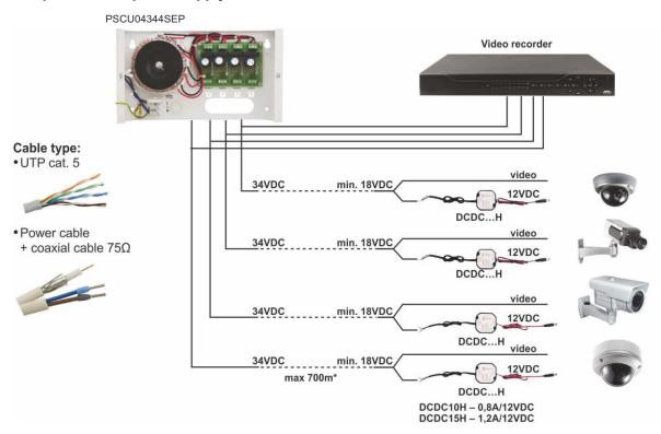
Typical distances between the power supply and the DC/DC converter:
