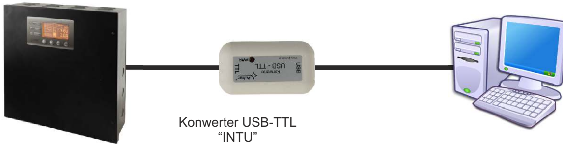
USB-TTL communication using the USB-TTL „INTU” interface.
