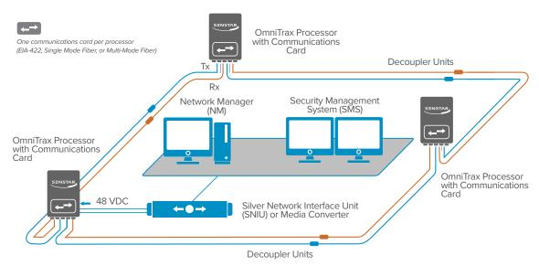
Note: No more than 5 processors may have their sensor cables electrically connected through decouplers (each group of up to 5 processors must have terminators installed at each end of the group). Data communication loops are extended across additional groups via group-to-group fiber-optic communication cables
