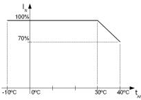
Chart 1. Acceptable output current from the PSU depending on ambient temperature.
