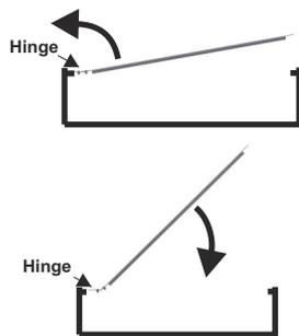
The enclosure is equipped with a hinged mounting plate max. 3 pcs.
